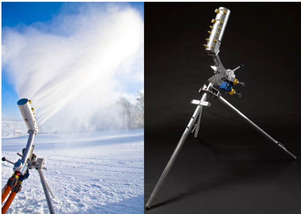
Figure 2. HKD Snowmakers' High Efficiency Viper Snow Gun. Source: Mark Horton, HKD Snowmakers.
