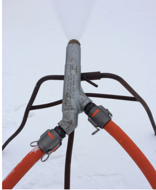
Figure 1. A typical, standard efficiency snow gun.
