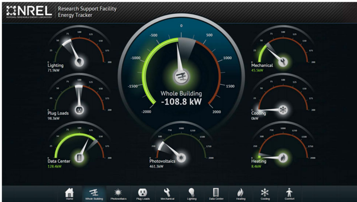
Figure 1. Building energy dashboard for NREL’s Research Support Facility with gauges for quick assessment of performance. Source: Pless 2015.
