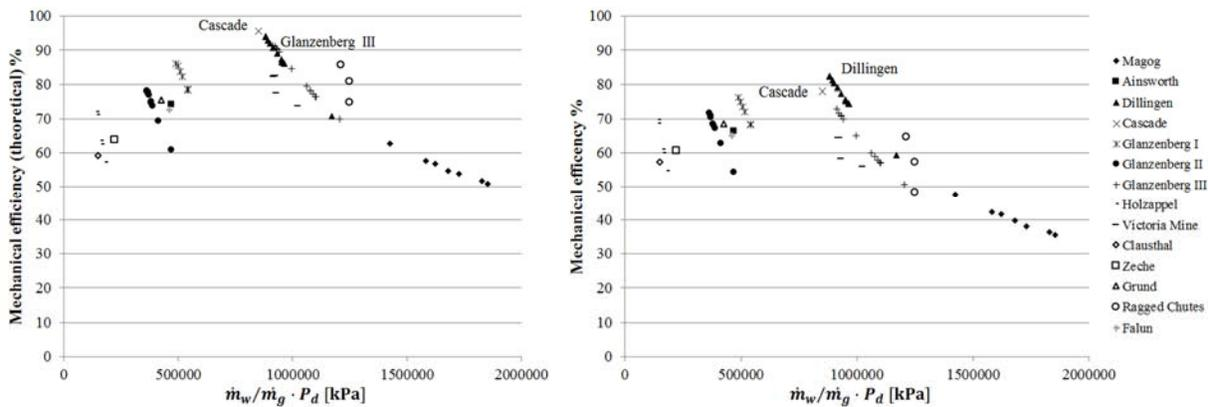
Figure 2. Theoretical and overall mechanical efficiency of 14 HAC installations, plotted against the product of mass flow ratio of the two phase (water, air) bubbly flow and delivery pressure.
