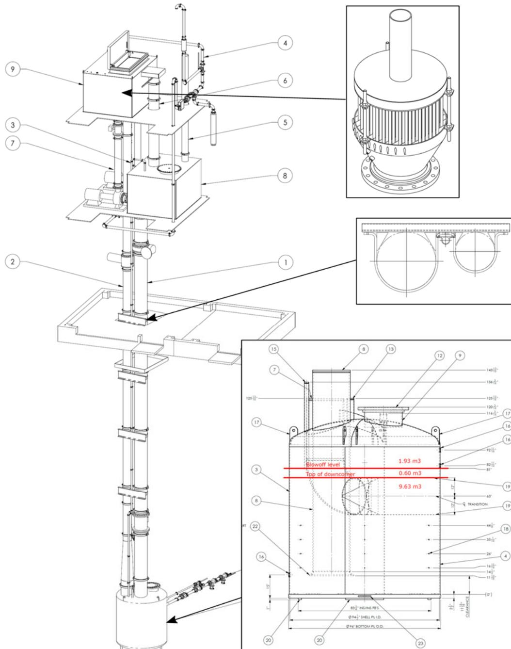
Figure 3. General arrangement of the HAC Demonstrator at Dynamic Earth, Sudbury, Ontario, showing detail of air-water mixing head in forebay tank (9), air-water separator and pipe bracket arrangements. 1- Riser pipe, 2- Downcomer pipe, 3- blow-off pipe, 4- Air intake, 5- tail race surge/vent pipe, 6- Spill-way pipe, 7- pump discharge pipe, 8- tail race tank.
