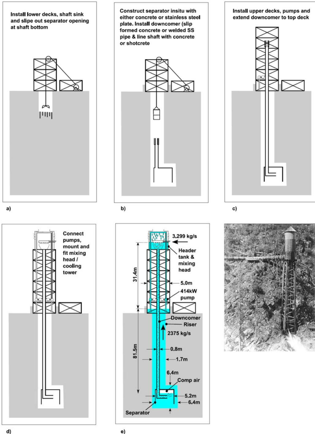
Figure 4. Construction sequence (a to d), process variables and design (e) of a 4700 Scfm HAC based on the Ainsworth / Kootenay installation (lower RHS). Note the design incorporating a cooling tower geometry as part of the header tank
