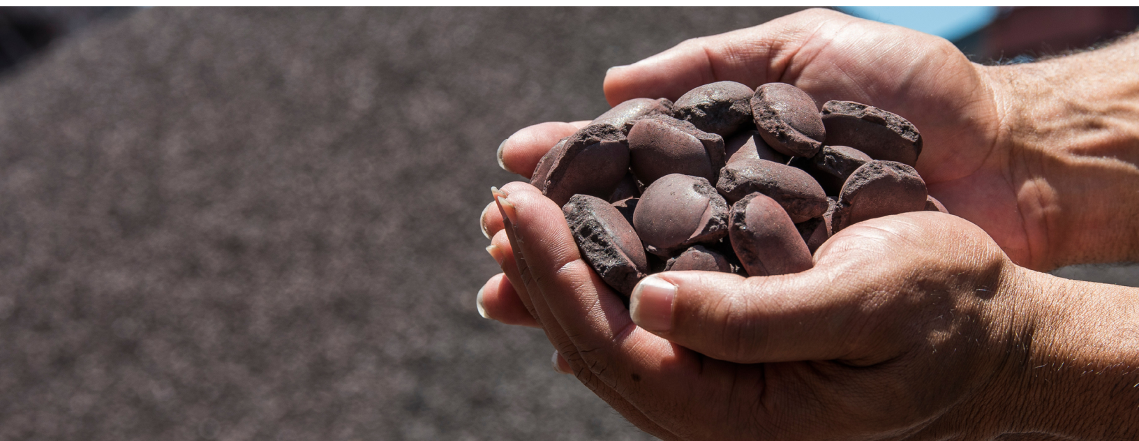
Cold-agglomerated iron ore briquettes (Photo by Gabriel Lordello)
