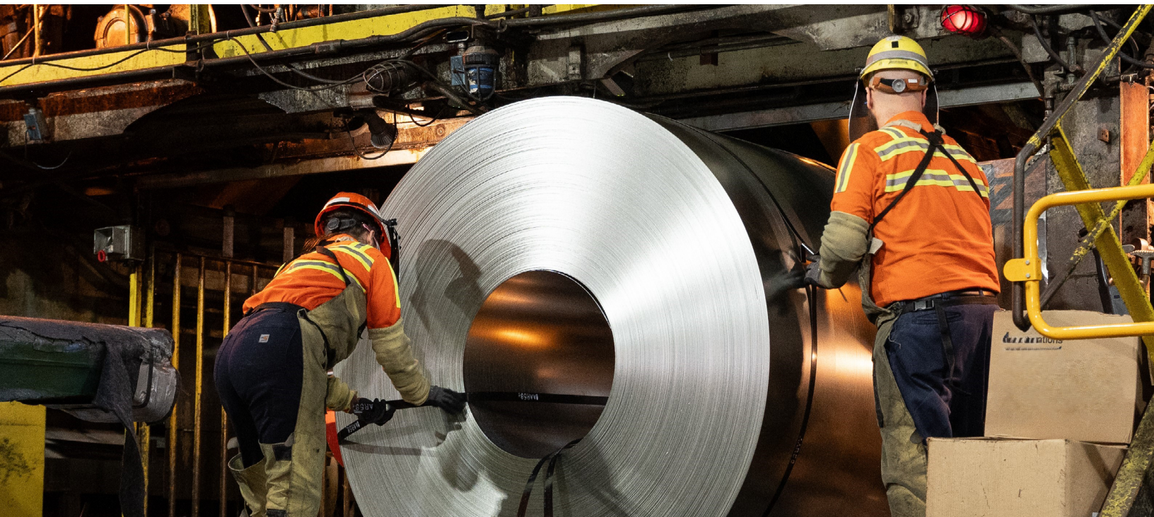
Middletown Works employees band finished steel coils
