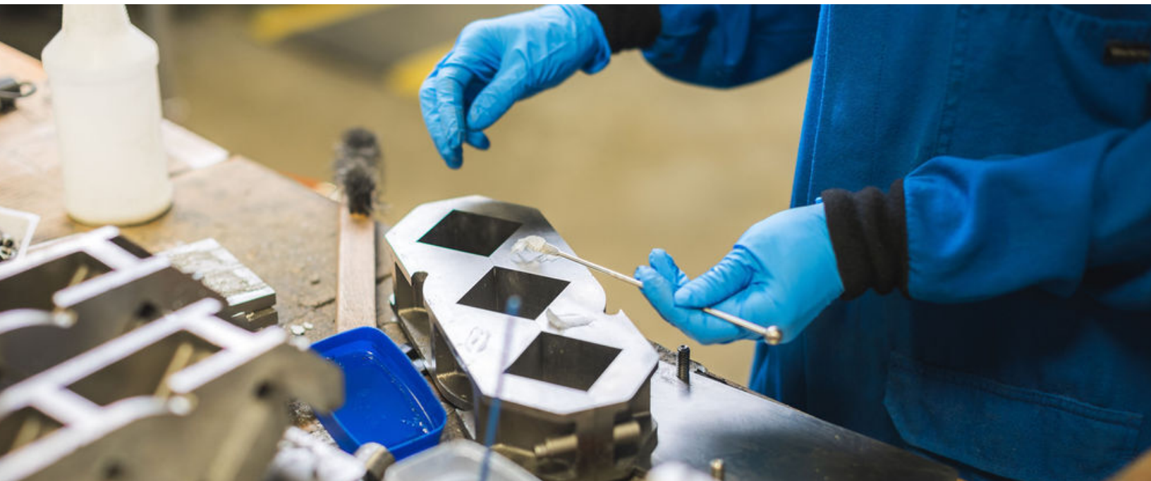
Brimstone prepares molds to cast samples using the company's deeply decarbonized cement
