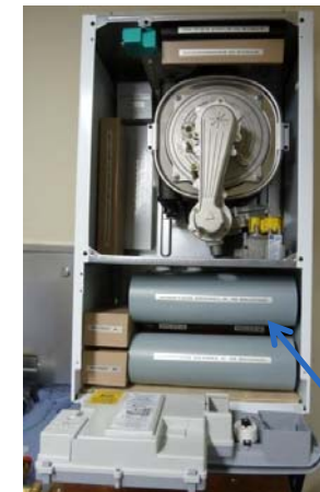
Adsorbent beds (generators)
