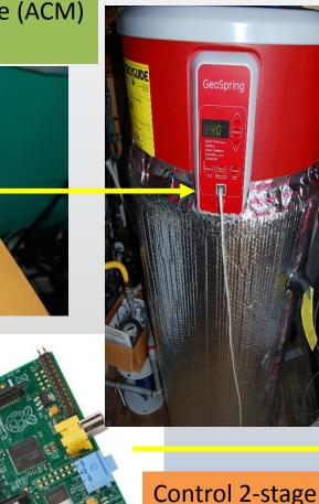
Determines Solar Electric production near real time and decide thermostat setting or element activation
