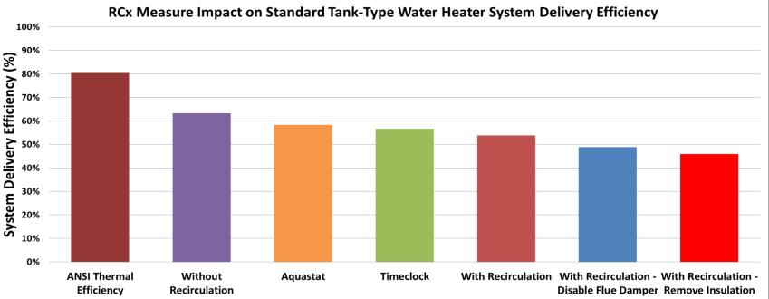
System Energy Performance Impact – RCx and Retrofit 24 hr. Draw Profile - Standard Efficiency Tank-Type Water Heater Insulated System
