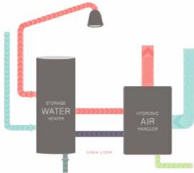
COMBINED WATER AND SPACE HEATER USING STORAGE WATER HEATER
