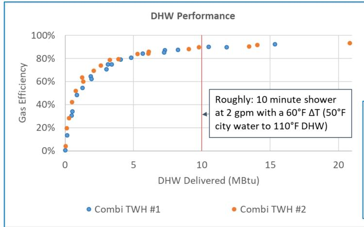
Like space heating efficiency, water heating efficiency depends on part-loads and can be characterized and predicted.
