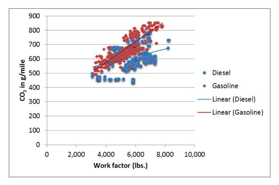
Figure 4. CO<sub>2</sub> emissions versus work factor for HD pickups and vans by fuel
