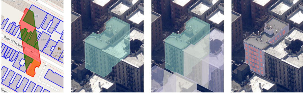
Figure 8: Example of selecting only relevant annotations (right) by identifying nearby building footprints (left), projecting the outline of the targeted building onto the image (center-left), then projecting adjacent buildings onto the image (center-right). Imagery source: Pictometry International Corp. Copyright © 2023. All Rights Reserved. Basemap source: NYC DoITT, OpenStreetMap.
