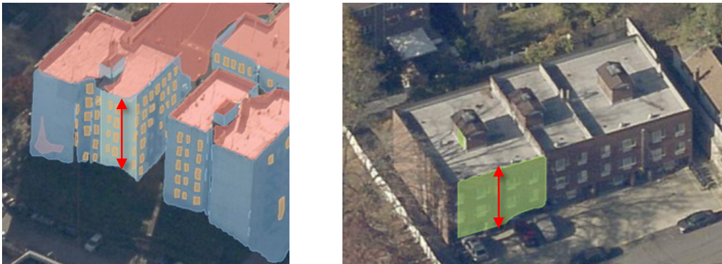
Figure 5: Examples of building height measurement using vertical cross-section detection. Imagery source: Pictometry International Corp. Copyright © 2023. All Rights Reserved.
