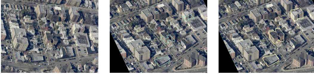
Figure 7: An original image (left) is first rotated to correct for sensor angle, next building footprints are projected onto the image (center), then translated to form a bounding polygon around each building. Imagery source: Pictometry International Corp. Copyright © 2023. All Rights Reserved.
