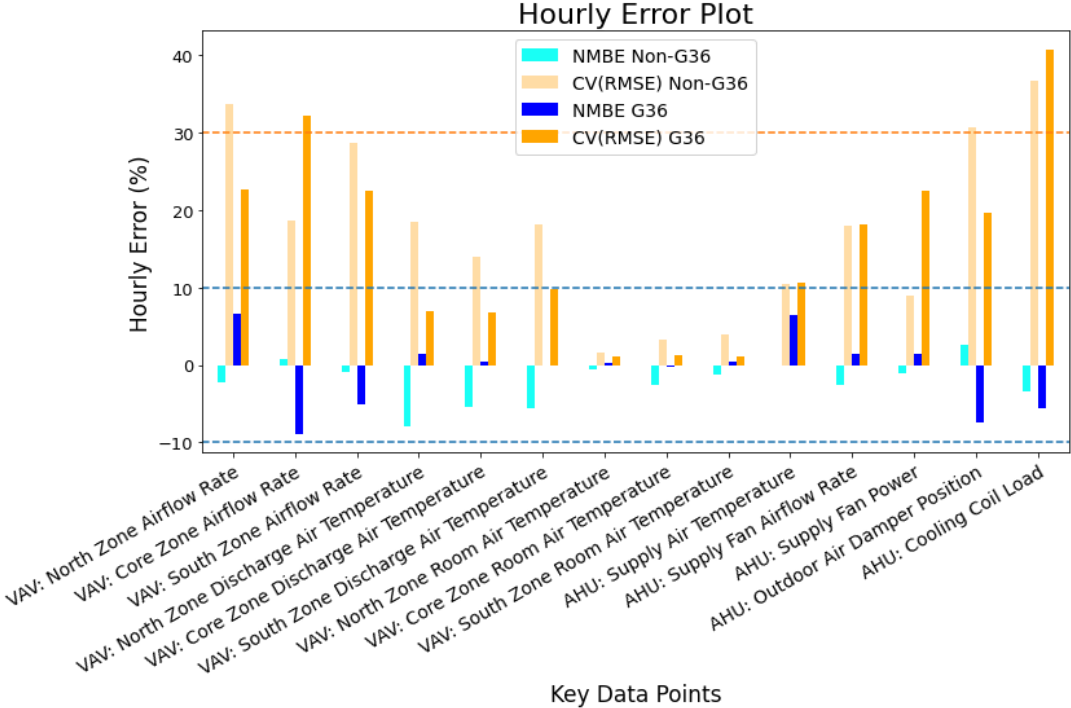
Figure 5: Overview of errors for 14 key data points considered in model calibration for the G36 and the no-G36 control sequences.
