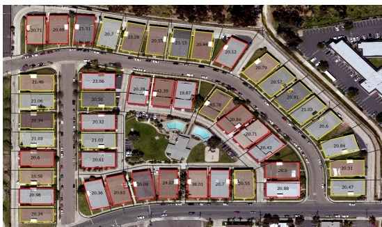
Figure 3: Satellite View of MF Complex with Roof Height Estimates
