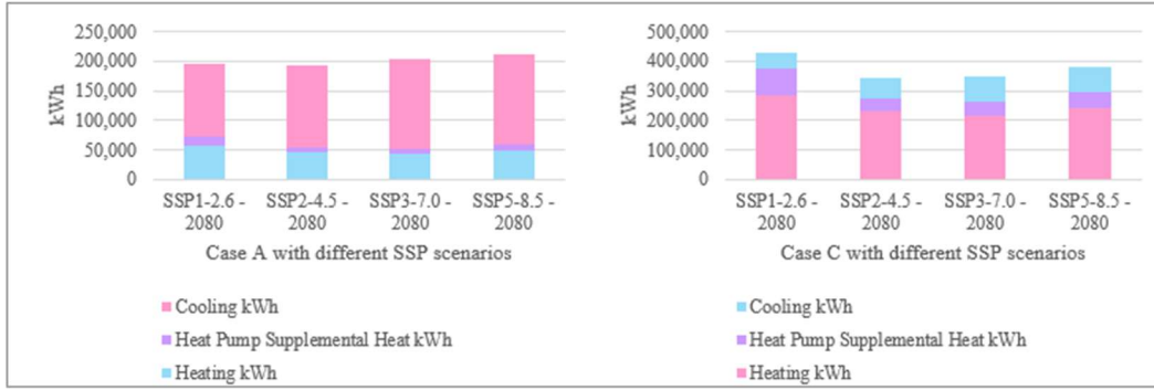
Figure 6. Heating, Heat Pump Supplemental Heat, and cooling between Case A and C – EPWshiftr file in the year 2080
