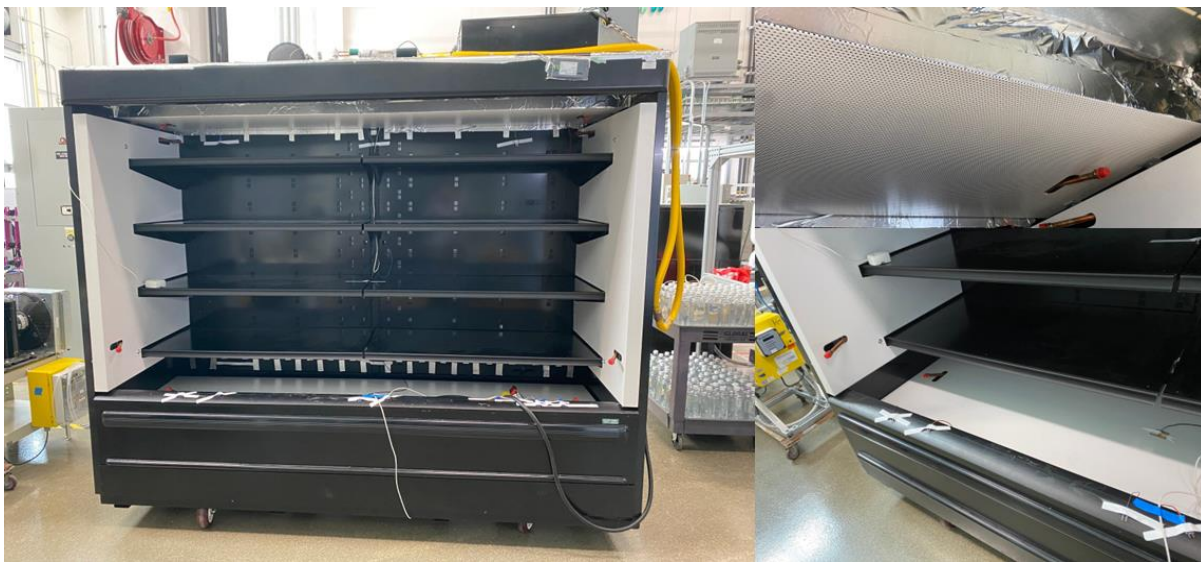
Figure 10. Images of the radiant panels (white surfaces) mounted to the baseline OVDC.
