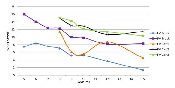
Figure 9. Energy savings from vehicle platooning. Source: Jootel 2013.
